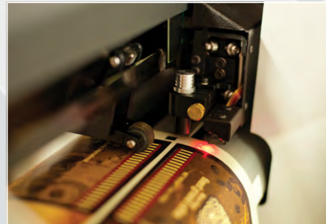
Optical sensors read up to 3 registration marks which ensure the best accuracy in the industry.
